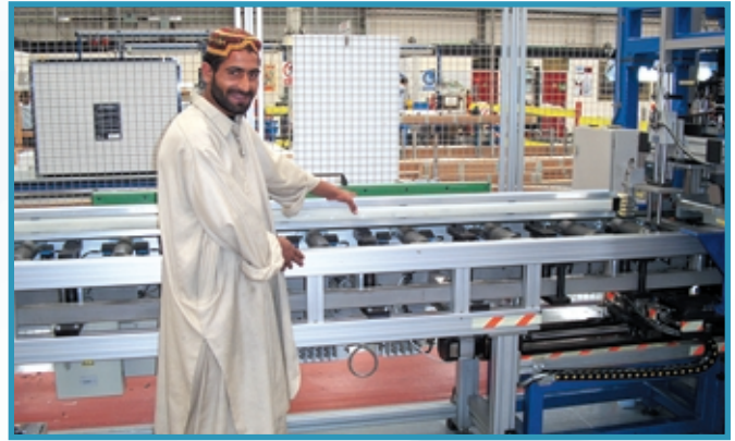
Automated riveting of bar sets
