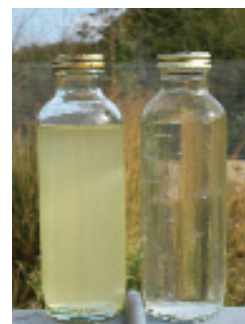
Contaminated water before (left) and after treatment in the wetlands
